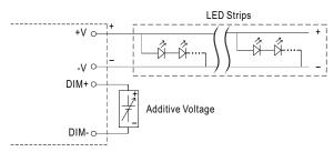
"DO NOT connect "DIM- to -V"
