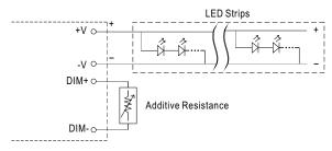
"DO NOT connect "DIM- to -V"
