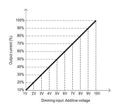
O Applying additive 10V PWM signal (frequency range 100Hz ~ 3KHz):
