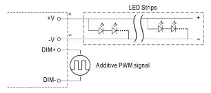
"DO NOT connect "DIM- to -V"
