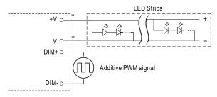
"DO NOT connect "DIM- to -V"
