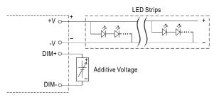
"DO NOT connect "DIM- to -V"
