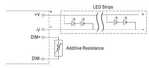
"DO NOT connect "DIM- to -V"
