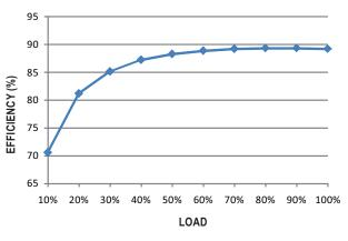
○ The curve above is measured at 230VAC.
